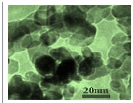
Fig. 1. TEM image of ZnO nanoparticle.
