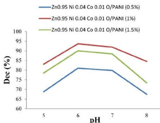
Fig. 5. Effect of concentration changes of  $Zn_{0.95}Ni_{0.04}Co_{0.01}O/PANI$  photocatalyst on decolorization activity at pH: 6
