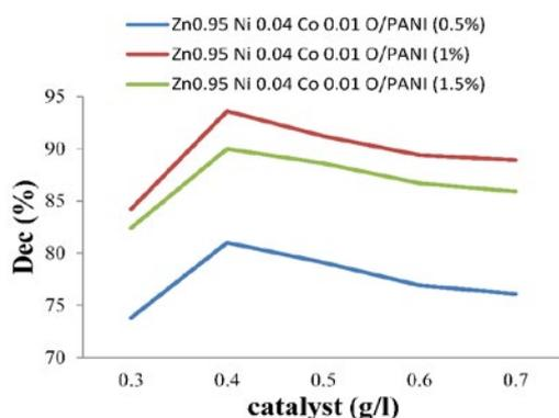
Fig. 6. Decolorization trend of 10 ppm in presence of  $Zn_{0.95}Ni_{0.04}Co_{0.01}O$ /PANI (0.5%, 1% and 1.5% PANI by weight) photocatalysts under light irradiation
