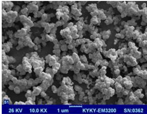
Fig. 1. SEM image of chitosan nanoparticles
