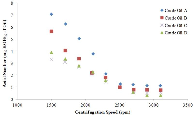
Figure 3: Variations of acidity of Iranian heavy crude oils vs. centrifugation speed.
