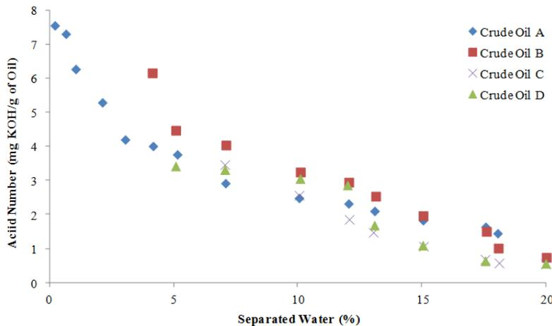
Figure 2: Variations of acidity of Iranian heavy crude oils with separation of formation water.
