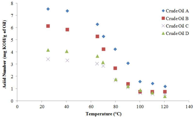
Figure 1: Variations of acidity of Iranian heavy crude oils vs. temperature.
