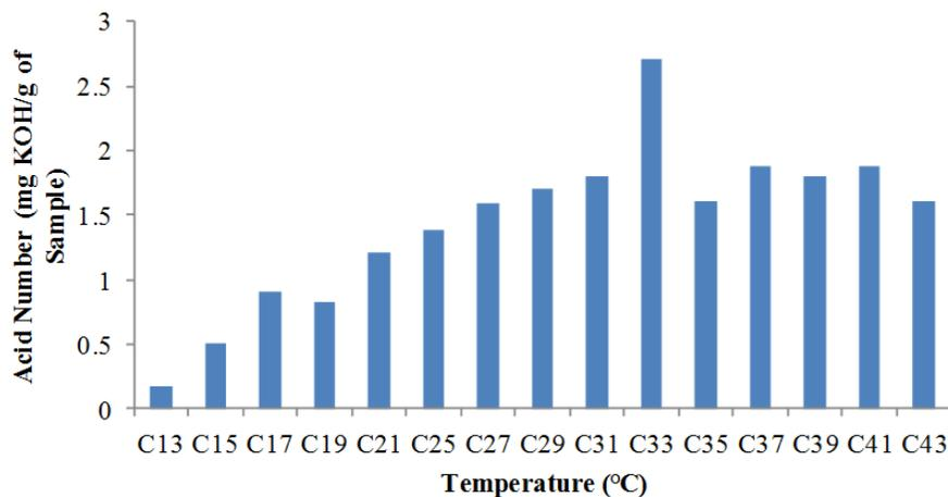
**Figure 4:** Distribution on acidity of crude A fractions.
